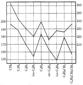
Upper curve: cracking temperatures of ethers  $(C_{\delta}H_{\delta})_{\delta}$ -C-OR; temperatures on the right side of plot. Lower curve: cracking temperatures of esters  $(C_{\delta}H_{\delta})_{\delta}$ -CCOOR; temperatures on the left side of plot. Fig. 1.
